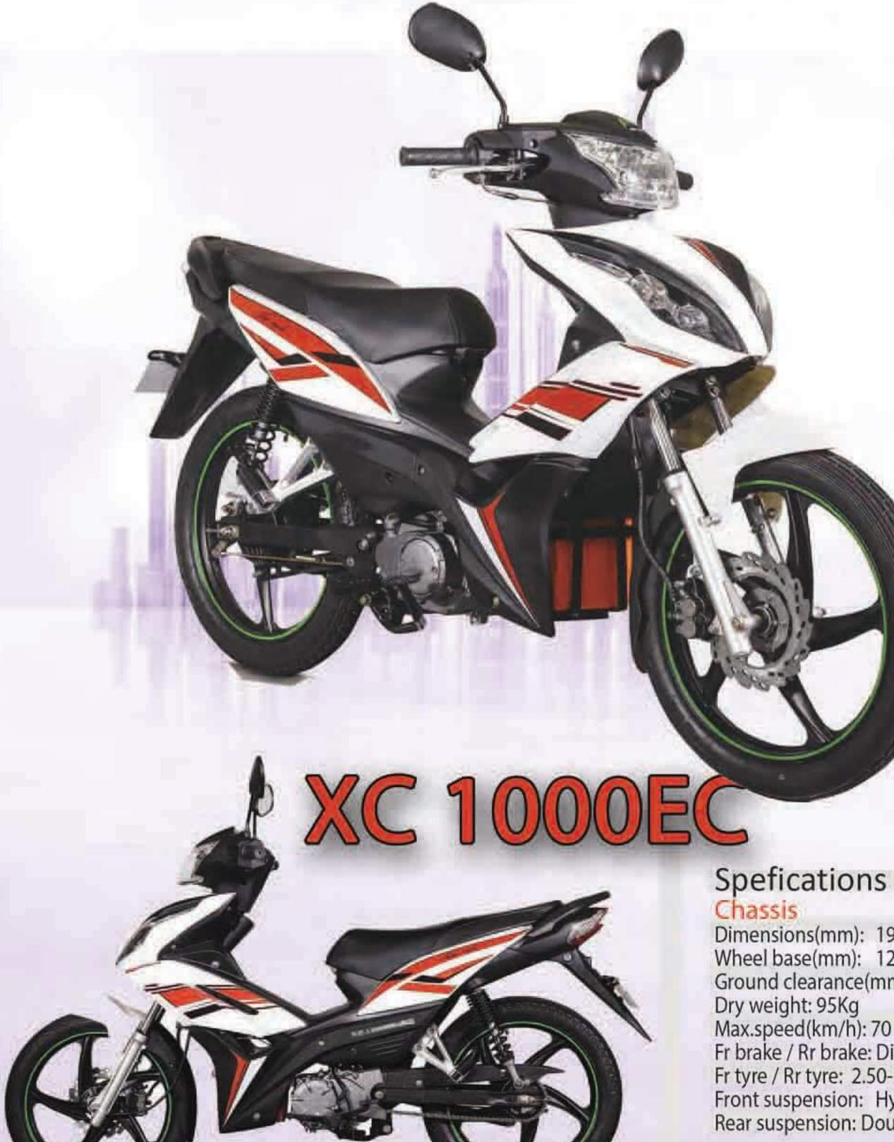
Dimensions(mm): 1900x700x1110 Wheel base(mm): 1250 Ground clearance(mm): 120 Dry weight: 95Kg Max.speed(km/h): 70 Fr brake / Rr brake: Disk / Drum Fr tyre / Rr tyre: 2.50-17, 2.75-17
